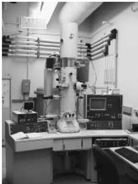
The recently installed high-resolution transmission electron microscope (JEOL-2010F FasTEM) in the CNM. This instrument is used to directly image the structure of a wide range of samples including Si nanocrystals, nanoparticle/biological composites, “quantum wires” and much more.
